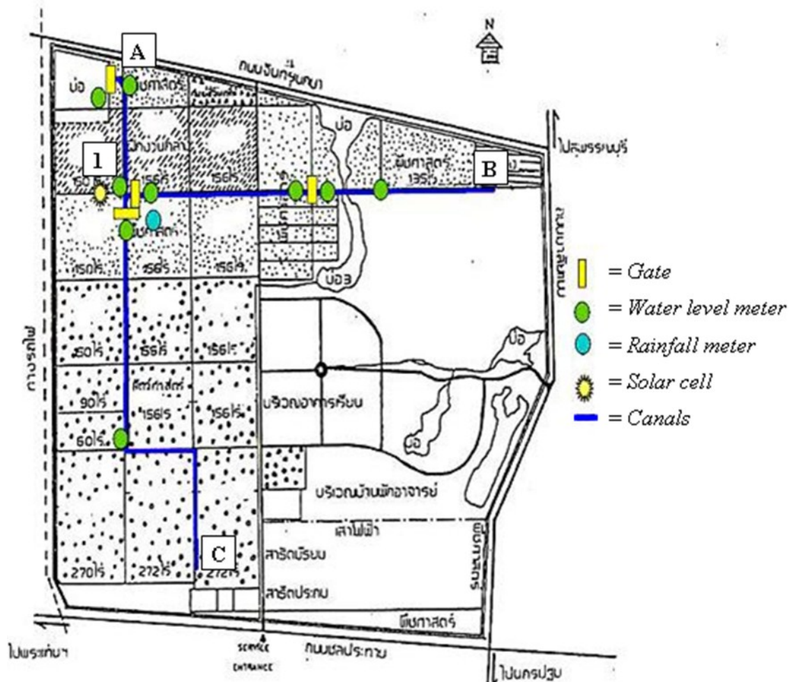
Figure 13: Model of a Water Gate System (Kasetsart University, n.d.)
