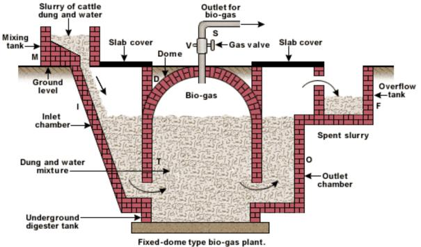
Figure 12: The Bio-gas Making Process
