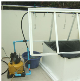
10. Unplug pump, close outlet valve, remove drainhose, and replace outlet hose. Turn pump on for approximately 10 minutes in order to flush nozzles. Insure bucket remains full of clean water.
