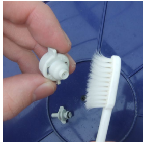
8. Clean nozzle cap with brush.
