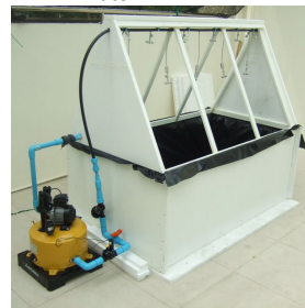
12. Replace top, replace screws in top, reconnect outlet hose, and reconnect check valve coupling. Follow nutrient solution mixture and planting procedures.
