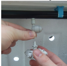
13. Replace nozzle assembly by pressing nozzle assembly into pressure sensitive valve.
