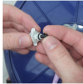
9. Remove jet from nozzle.
