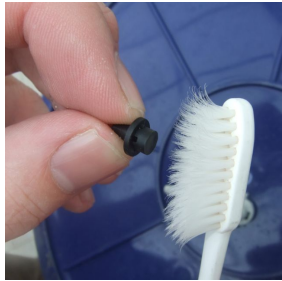
10. Clean jet with a brush, if needed a pin can be used to clear clog.
