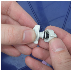
7. Remove nozzle cap.
