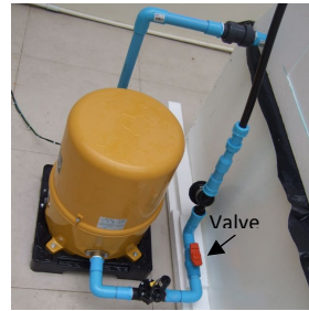
12. Plug pump in, open outlet valve and let pump run for at least an hour to completely circulate and mix nutrient solution.
