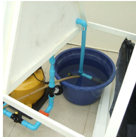
8. Lift top up, slide forward, and place pump inlet into a full bucket of clean water.
