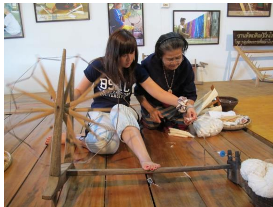
Figure 4.3.1-1 A photograph, taken at the Haad Siew Weaving Center, illustrating the ‘ Khen Fai ’ or traditional cotton spinning process
