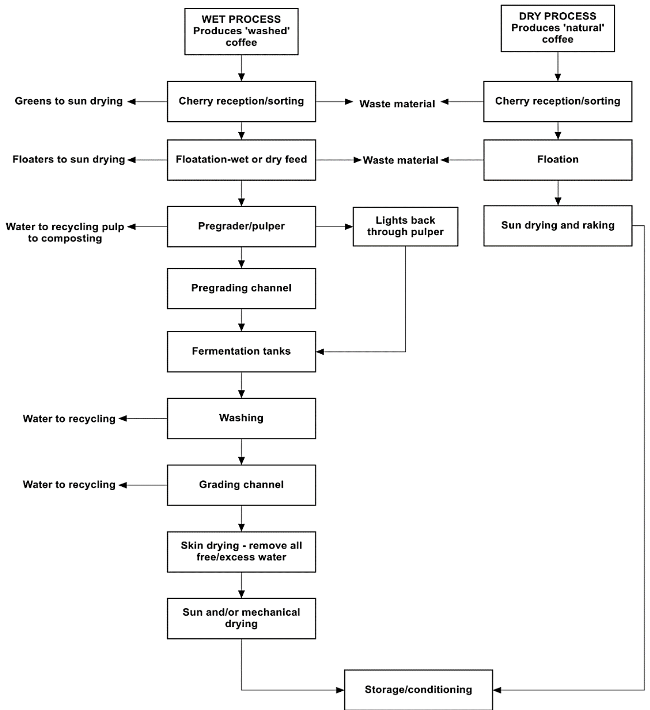
Figure 2.6 The diagram of wet and dry processes (Sabtu, 2012).
