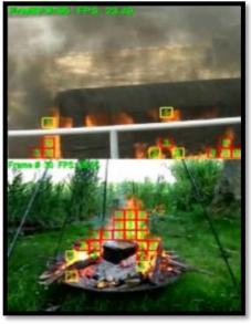
Figure 13: Video Analytics software detecting fire (http://signal.ee.bilkent.edu.tr/VisiFi
