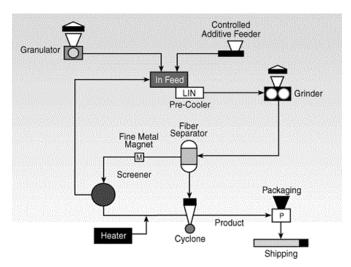
Figure 10 - Cryogenic Grinding Process (Tire Recycling Made Simple, 2012).
