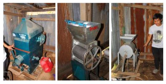
Figure 5: Various Machines Used for Pulping, Hulling and Polishing
