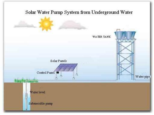
FIGURE 13: SOLAR WATER PUMP SYSTEM FROM UNDERGROUND WATER (IDA-TECH, 2011)
