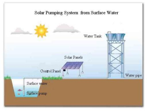
FIGURE 14: SOLAR PUMPING SYSTEM FROM SURFACE WATER (IDA-TECH, 2011)
