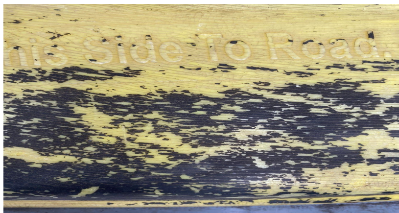
Figure 12: The garbage bin has been corroded by solvent
