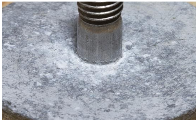
Figure 30 : An aluminium part that has oxidized
