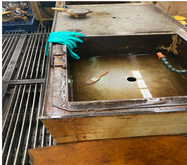
Figure 27: The poor condition of the washing bench with scraped paint and rusty.
