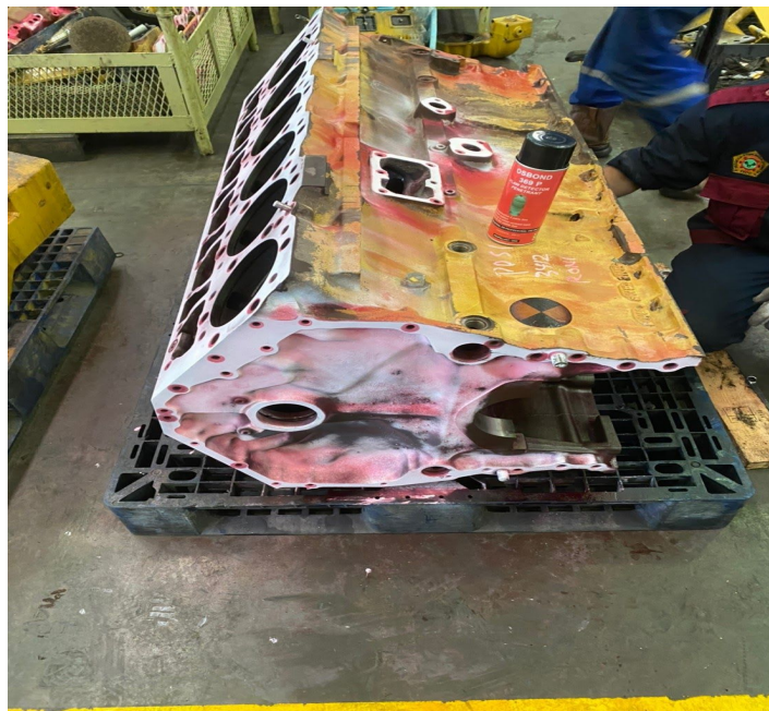
Figure 22: Machine was painted in the white-red color to detect hairline fractures
