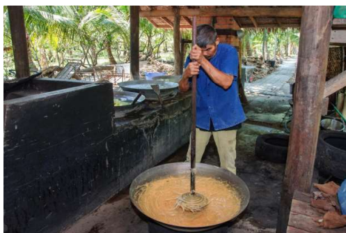
Figure 2.2 This picture shows one of the coconut sugar making process. Staff is foaming up the sugar to add air pocket using device resembled egg beater.
