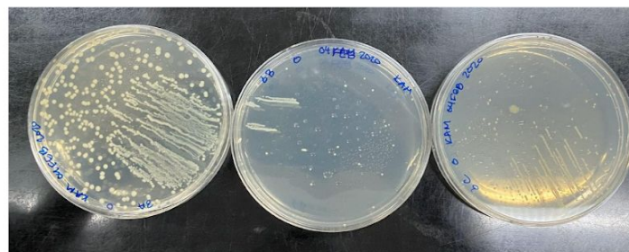
Figure 23. From left to right: Source, pre-filter and point of use bacterial contamination at the Ban Mae Salap school. All plates non-diluted, 100 \mu L water sample incubated at 36°C for 24 hours.
