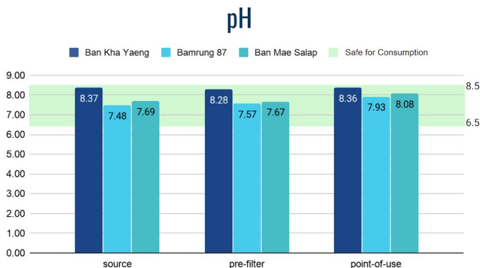
Figure 20. Changes in pH at each point in the drinking water system at three schools. Water below the value of 6.5 or above the value 8.5 is not safe for consumption.
