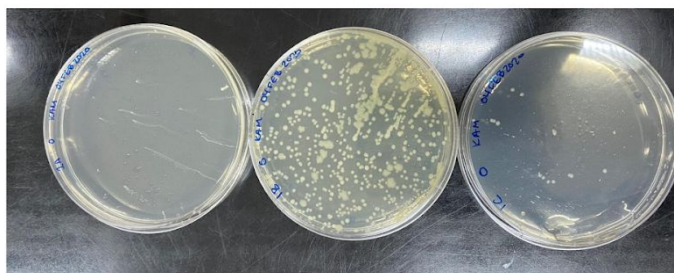
Figure 21. From left to right: Source, pre-filter and point of use bacterial contamination at the Ban Kha Yaeng school. All plates non-diluted, 100 \mu L water sample incubated at 36°C for 24 hours.
